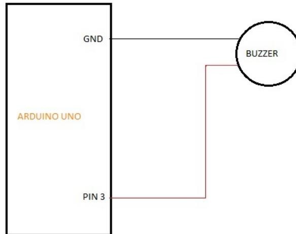
**Fig.1 Connection Diagram for Interfacing Buzzer With Arduino**
