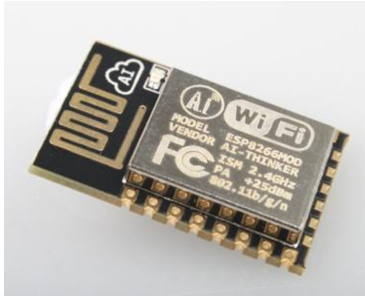
Figure 3 [Module Pin Counts, 22 pin, 16 mm *24 mm *3 mm]
