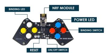
• First, we have to connect the NRF Module. Otherwise status LED BLINK Continuously.
