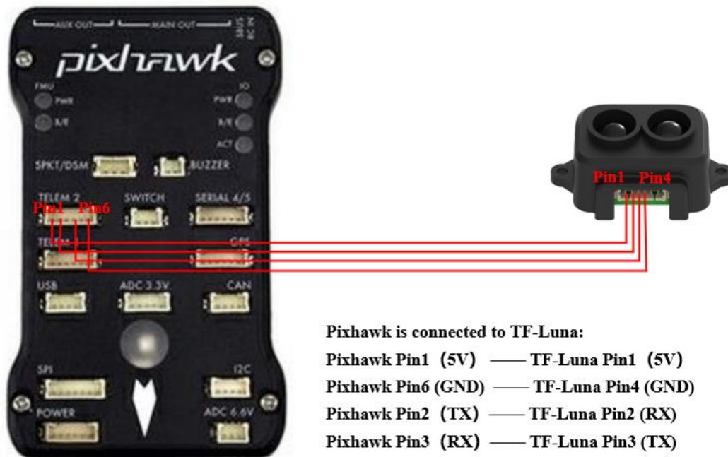
Figure 1 Schematic Diagram of Connecting TF-Luna with TELEM 2 Interface (Serial Port 2) of Pixhawk
