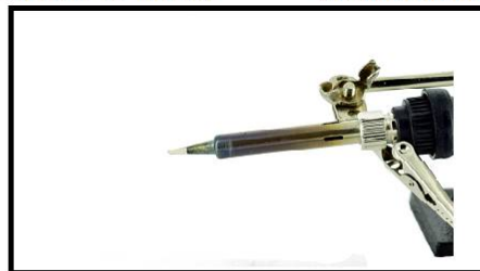
3. PROPERLY TINNED SOLDERING IRON TIP
