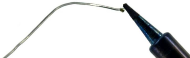
3. PROPERLY TINNED SOLDERING IRON TIP
