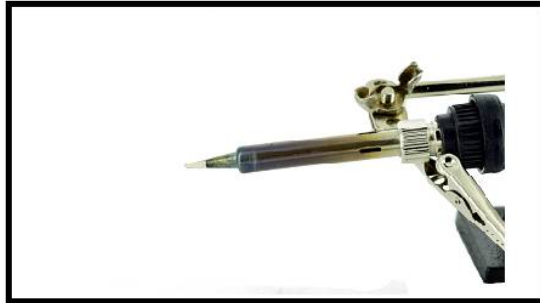
3. PROPERLY TINNED SOLDERING IRON TIP
