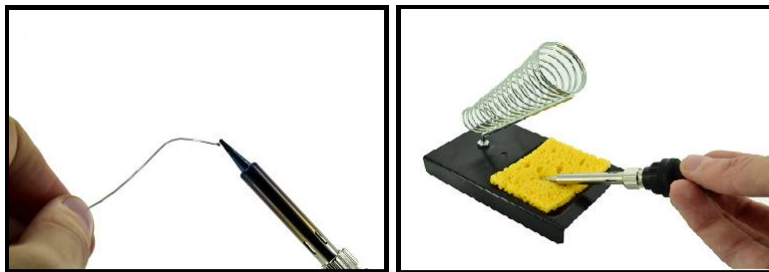
1. APPLY SOLDER TO THE TIP
