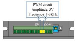
RV should be rotated anticlockwise Notice to limit position.
