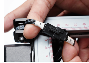
Y(4PIN)→Y-axis Stepper Motor Cable
