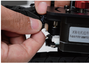
X(4PIN)→X-axis Stepper Motor Cable
