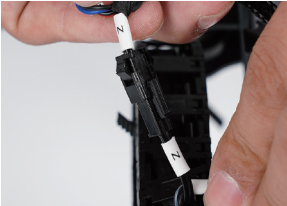
Z(2PIN)→Z-axis Endstop Switch Cable
