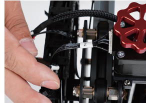
Z(4PIN)→Z-axis Stepper Motor Cable
