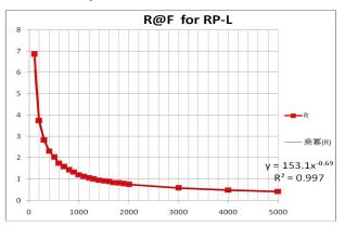
The following plot shows a near-linear curve whose axes value treated by log10.
