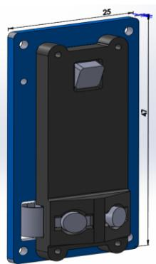
GS5 provides ZH1.5-4P receptacle, which has system power supply and data communication interface.
